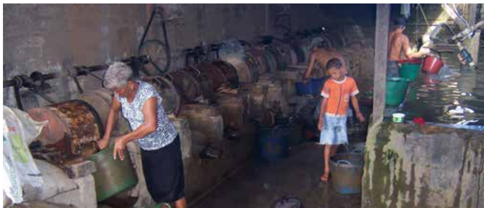
WOMEN AND CHILDREN GRINDING THE ORE WITH MERCURY INTO SMALL BALL MILLS
